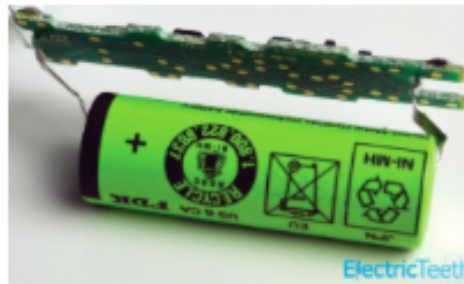
Figure 5: Ni-MH rechargeable battery (Love, 2016)
