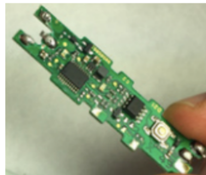
Figure 8: Oral-B Pro 1000 Mother (Circuit) Board (Kinsey, Tolbert, & Suovanen, 2017)
